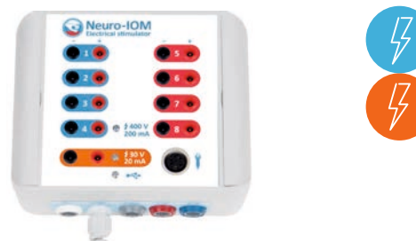
9-channel Neuro-IOM electrical stimulator unit Application: generation of high-amplitude stimuli via 8 independent channels and low-amplitude stimuli via 1 channel during surgery
